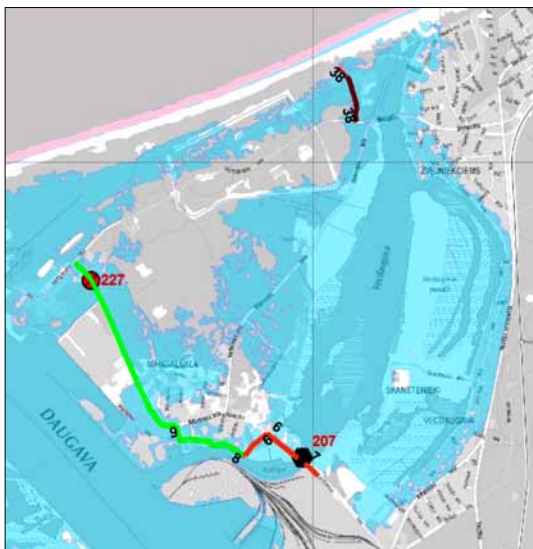
Fig. 4. Flood protection location (a sluice system) in the Vecdaugava River neighbourhood, the 1st case (Plūdu riska 2010)
