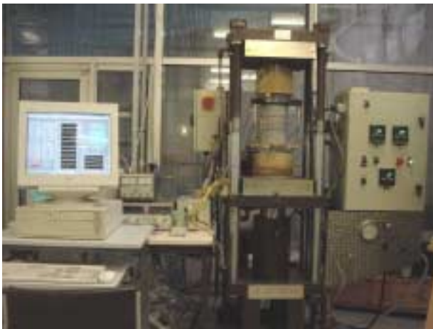
Fig 2. General view of the test device for transient thermal test of concrete
