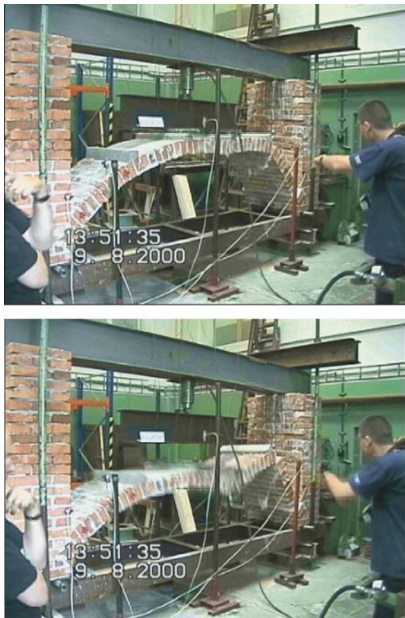
Fig 3. Vault failure under load (buckling of right vault section)
