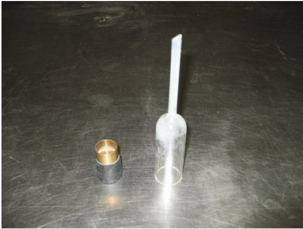
Chase indicator used for determining the air content of mortars
