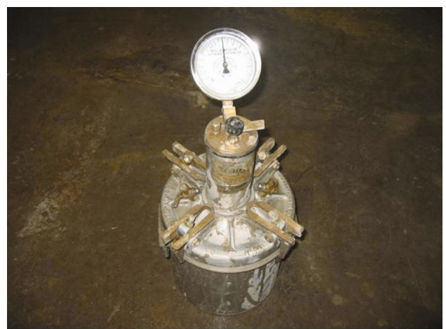
Measurement of concrete air content
