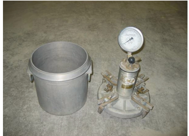
Type B air meter used for determining the air content of concretes
