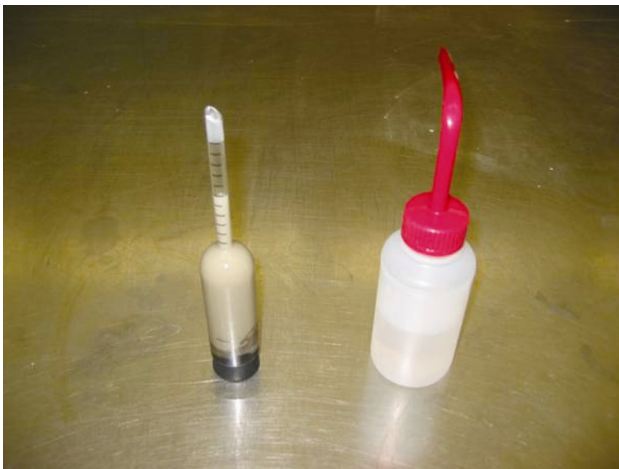
Measurement of mortar air content
